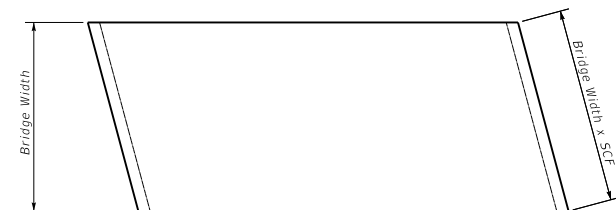
PLAN OF SUPERSTRUCTURE SLAB
